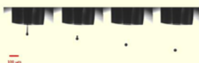
Figure 3: Stroboscopic control image of a drop formation through a dispenser nozzle. Every image has been taken with an interval of 100 μs.
